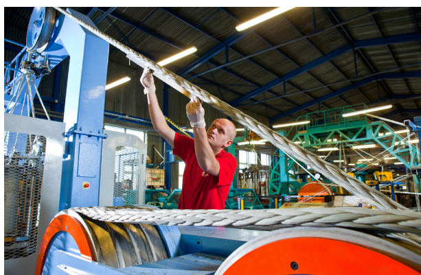
Figure 2. During production, it is important to do quality checks to make sure that a high realisation factor is kept. The realisation factor is an important part of identifying how much strength of the original fibre is kept in the final rope design.
