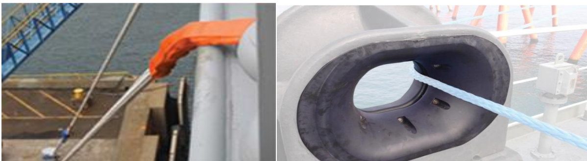
Fig 16: Mooring Line chafe protection.
