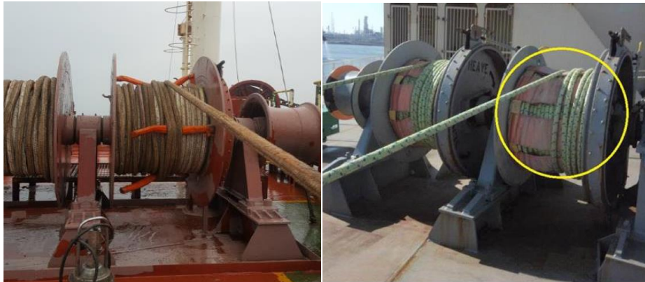
Fig 15: Anti mooring Line embedding
