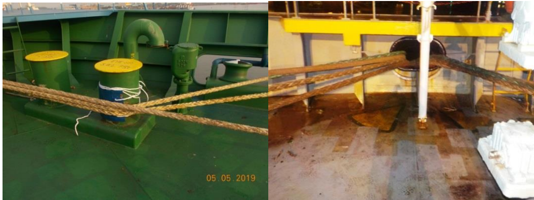
Fig 13: Overloading Fairleads and mooring bits (source Anglo Eastern)
